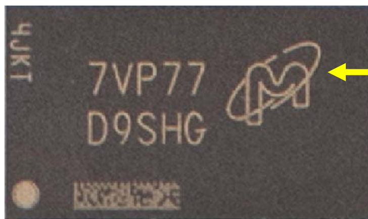
Figure 2 – Unaffected Module with Micron DDR Identified with the Micron M Logo
