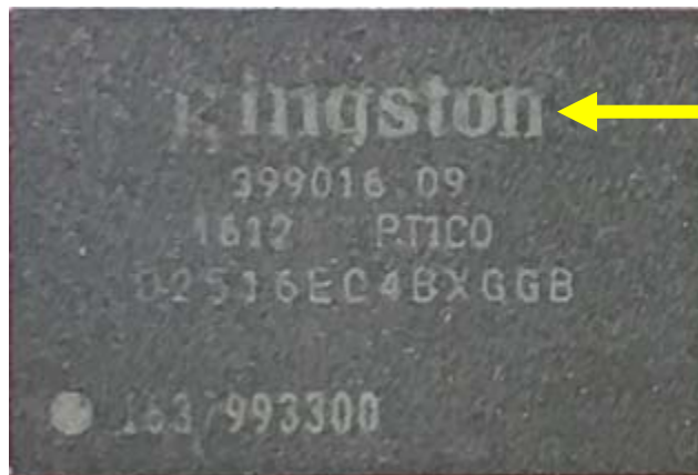
Figure 1 – Affected Module with Kingston DDR Identified with “Kingston”
